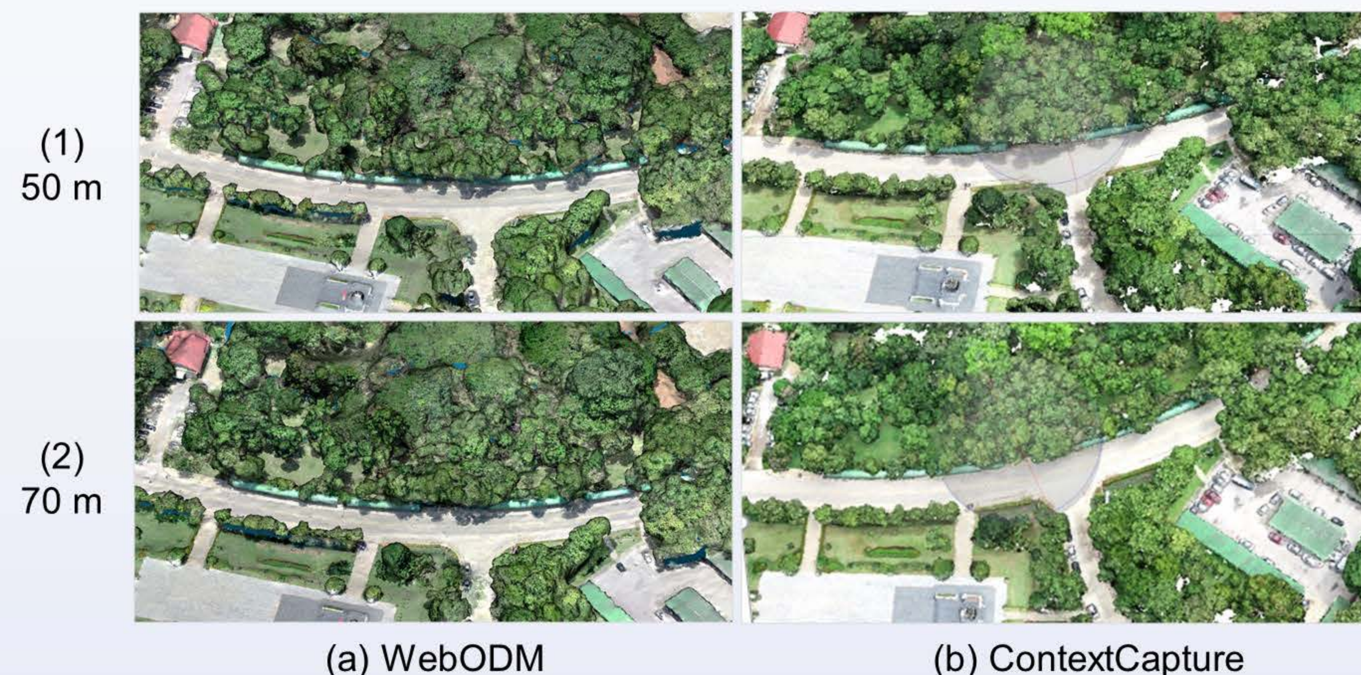
Figure 3. The 3D models obtained from (a) WebODM, and (b) ContextCapture using the UAV flying height at (1) 50 meters, and (2) 70 meters above the ground.
