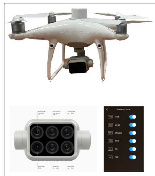
Figure 4 Phantom 4 Multi-Spectral Camera with RTK
