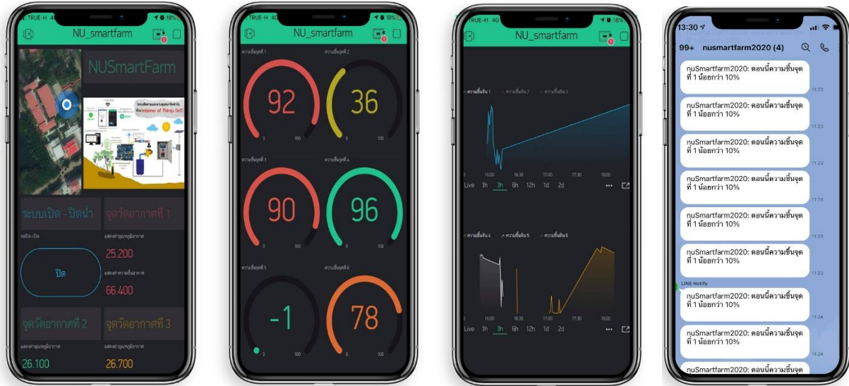
Figure 6 a-c is a Real-time soil moisture monitoring dashboard based on Blynk Application and (d) is LINE notify system
