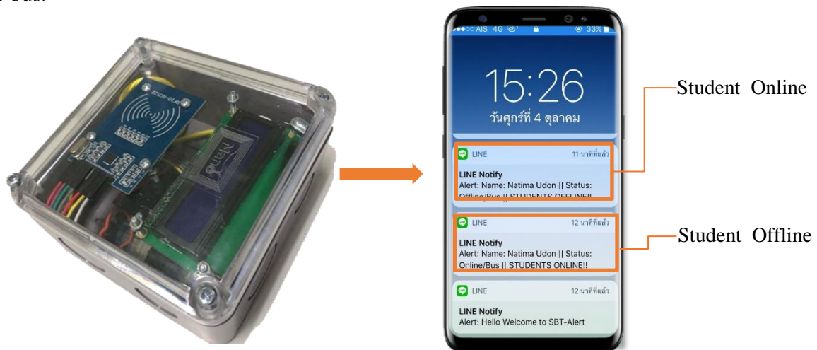
Figure 5 RFID Viewing Alert System
