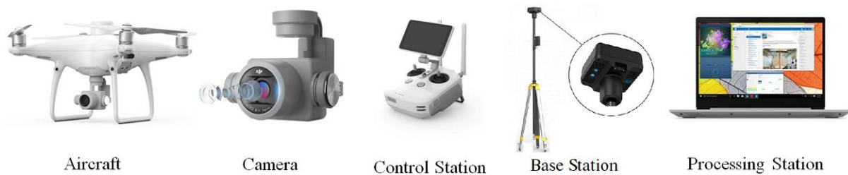
Figure 3. Phantom 4 RTK unmanned aerial vehicles (UAV) system
