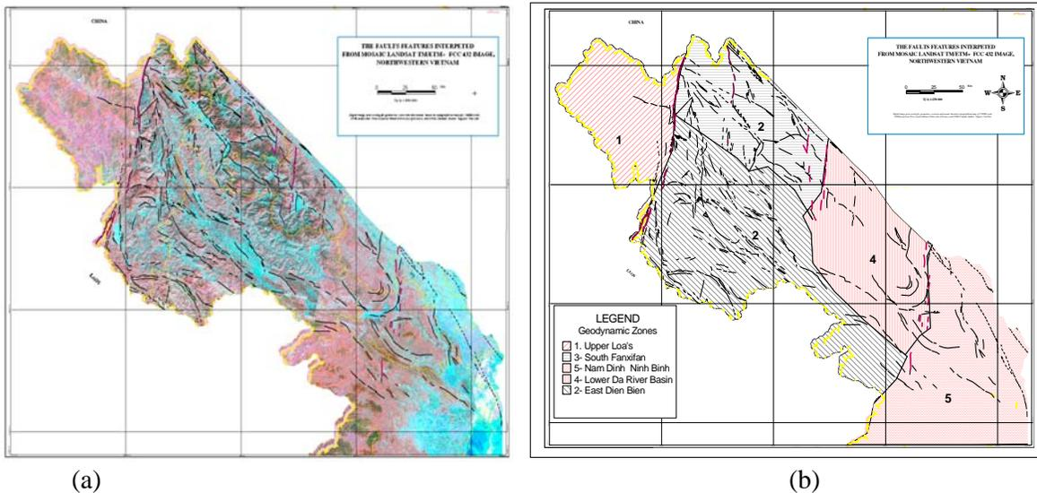
Figure 4. Faults displayed on FCC 432 Landsat images (a). Image interpretation of fault lines and geodynamic zones (b).
