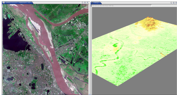
Figure 10. Sample data (left; ASTER image, right; SRTM data)
