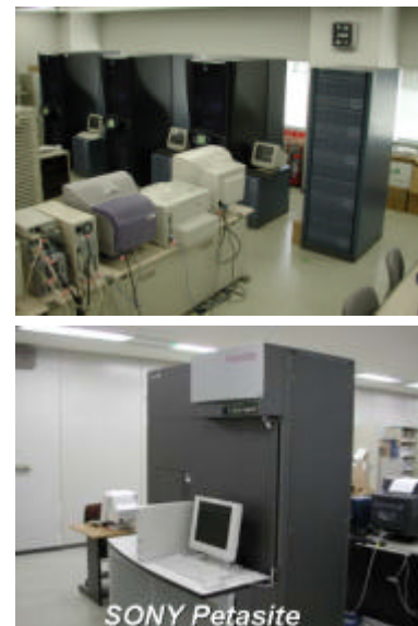
Figure 3. Picture of PALSAR GDS. (Top) Parallel computer system. (Bottom) Tape archive library(140TB).
