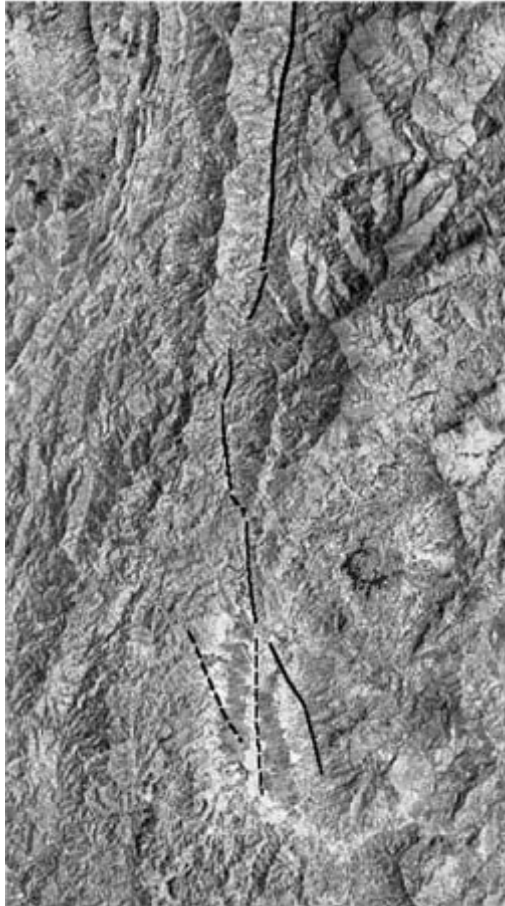
Figure1: Dien bien fault determined from LANDSAT image
